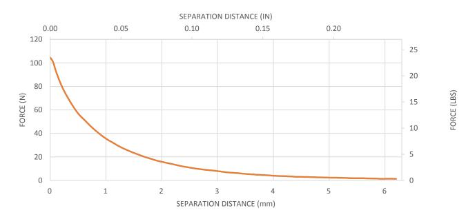
These Polymagnets provide very strong attachment forces to steel or their mating Polymagnet over their effective range compared to conventional magnets. These magnets are suitable for use with a metal target or another 1000324. The holding strength for these Polymagnets can be enhanced in many applications by using a thin steel shunt directly against the back of the Polymagnet, and this shunt will also help limit stray fields from the magnet.
